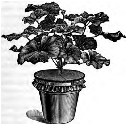
FIG. 28. — Aluminum shell, roofed with rubber, for preventing evaporation from soil and pot; \times \frac{1}{4} .
